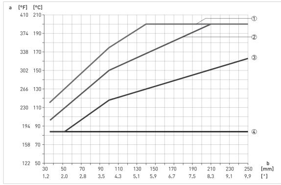
Figure 3-2: Media temperature versus external length of sliding connection
