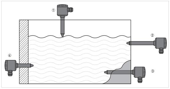
Figure 3-1: Possible applications for sliding connection
