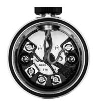
A Teach-In is necessary when the dielectric constant  $\{\epsilon_r\}$  is < 2 or a medium is hard to detect as present or not, e.g. when yogurt stick to the sensor tip. Teach-In can be done directly with the product by using the teach terminals in the housing.
