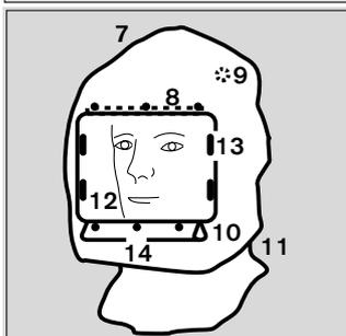
Suleika II is an open facepiece which can be "breathed over", i.e. adequate protection can no longer be guaranteed if the air supply deteriorates or fails completely. It must therefore **not be used** in the presence of carcinogenic, highly toxic or radioactive substances, microorganisms (viruses, bacteria, fungi and their spores) and enzymes, nor if there is a shortage of oxygen in the ambient air.
