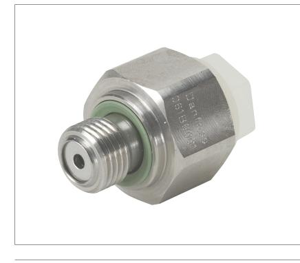
The MBV 2000 isolation valve is designed for mounting between Danfoss pressure transmitters with DIN 3852 - E pressure connection and fluid-filled systems.
