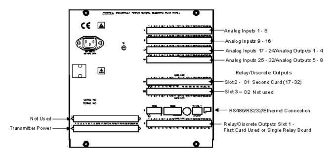
90 – 250 Vac Rear Panel AC power is connected via the standard configuration IEC chassis plug on the rear panel
