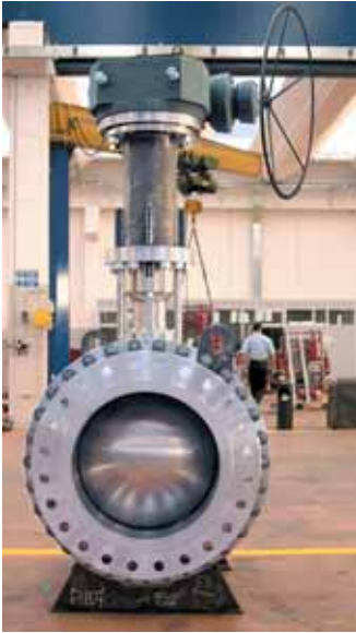
24" (600 mm) class 300 side-entry for high temperature.
