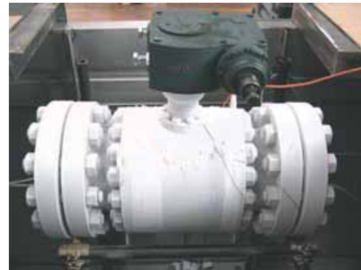
Cryogenic testing on an 8" (20 mm) class 300 valve.
