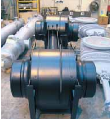
Fully welded 48" (1200 mm) class 600 for underground service.
