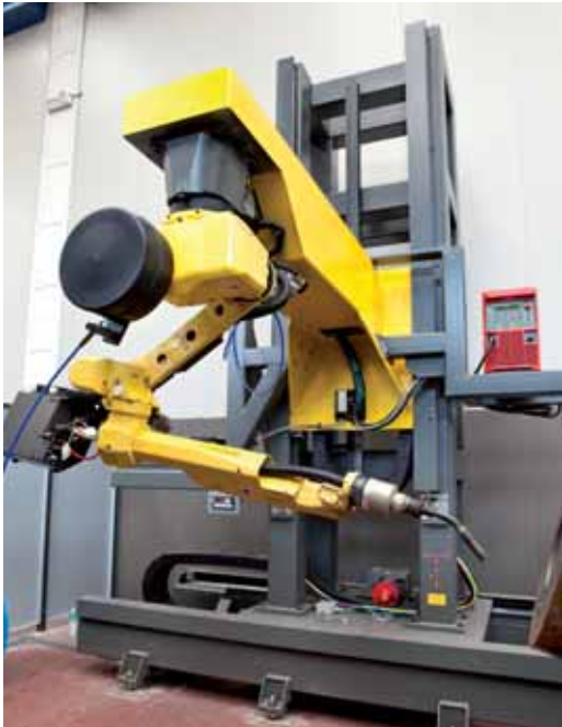
SAW welding robot applying weld overlay on valve closure
